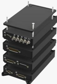
The Recorder, Integrated Processor, and Router (RIPR) series delivers flexible, low SWaP solutions for temporary or permanent sensor data acquisition, recording and streaming on mobile platforms. Any-to-any data routing, video compression, combined with precise packet timing simplifies data analysis, while open standard data formatting prevents vendor lock and enables AI-driven analytics.
