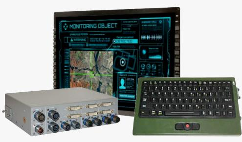
Spectra provides a wide range of rugged LCD displays for ground vehicles in various sizes ranging from 5.0" to 43", including sunlight readability and NVG compatibility. Various standard options include bezel keys, cold start capability and rugged AR touch screens. Additionally, Spectra offers a suite of rugged peripherals, including NIAP-certified KVM switches and keyboards.
